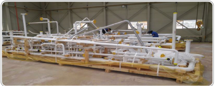
Manufacture of Pipe Spools
